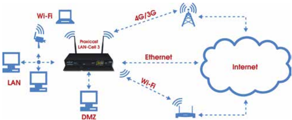
Figure 1: Typical LAN-Cell 3 Network Configuration
