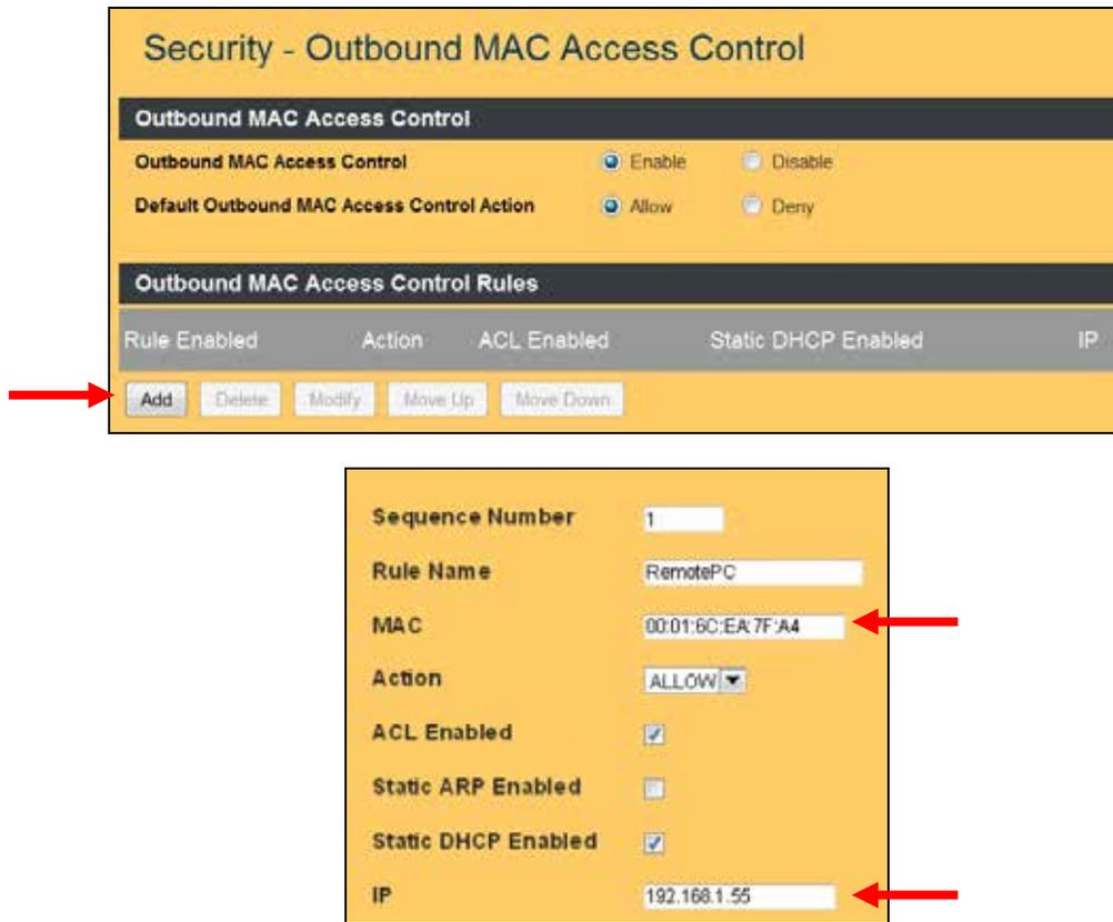
Figure A-2: Static DHCP Addressing in the LAN-Cell 3
