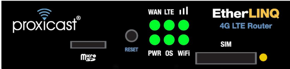
Figure 1: EtherLINQ Front Panel
