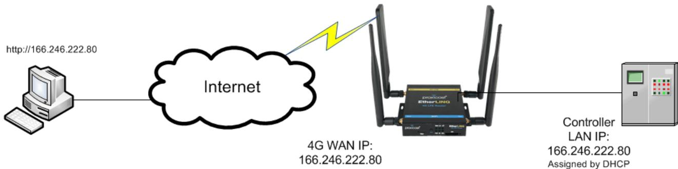
**Figure 17: IP Pass-Through Mode Example**
